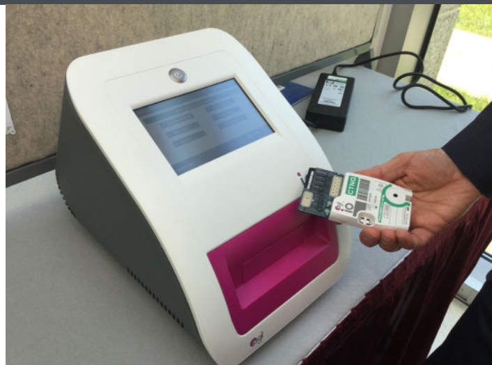
Above, the PhotoniCare device shows both the eardrum and the middle ear, making it easier for physicians to diagnose ear infections. Below, the ATLAS device is small enough to fit in a physician's office or at a pharmacy and can diagnose infections such as chlamydia and MRSA in minutes.
