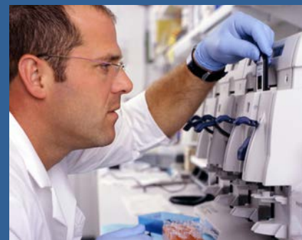
ON THE COVER: Biologist James Balow Jr. inserts a GeneChip into the GeneChip fluidics station to analyze RNA from patient samples in order to identify genes that are differently expressed between patients with autoimmune diseases and controls.
