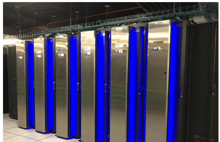
Biowulf is one of two supercomputers at NIH that Tolia used to run his calculations. Pictured here are the coolers used to keep Biowulf’s 99,000 computational cores at an appropriate temperature.
