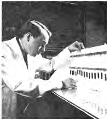
Joseph Foley separates hexosamines from interfering substances by means of cation exchange columns.
