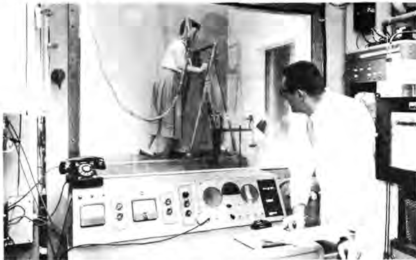
Ronald H. Thompson, physiologist in NIAMD, collects data on the energy expenditure of a normal control patient as she exercises on the treadmill in the metabolic chamber.
