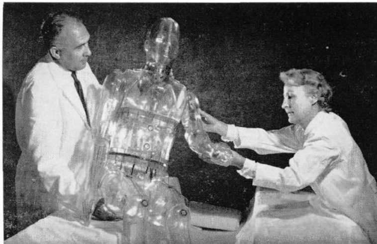
A transparent manikin, "Christine," is lowered into the U-shaped trough of the Clinical Center's new whole-body radiation counter by Dr. Howard L. Andrews, NIH Radiation Safety Officer, and his assistant, Dorothy Peterson. Eighteen gamma ray counters, concealed by the sheet covering the trough, will detect and locate radioactive material in Christine's "body."—Photo by Jerry Hecht.
