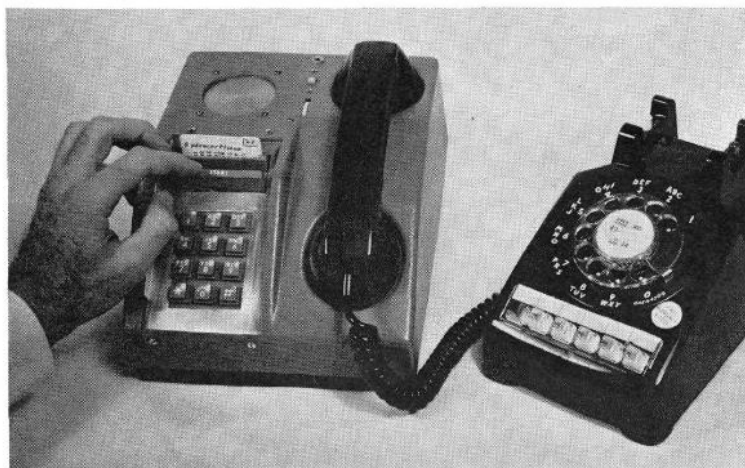
When the portable pushbutton pad is used to convert a dial telephone to a computer terminal, the telephone hand set is placed above the coupler as a receiver. The pad, powered by alternating current or battery, can be carried anywhere and linked to any telephone.
