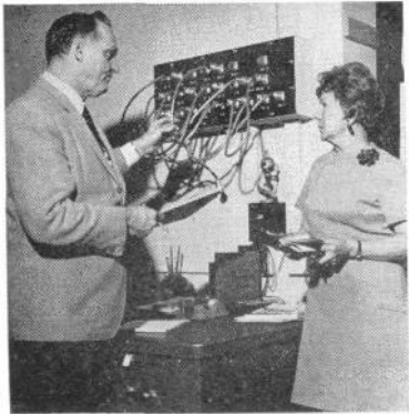
Transcriptions of meetings are fed back into Mr. Hollingsworth's remote control studio. He and Mrs. Meyer test the patch panel that controls the consoles placed in every conference room.
