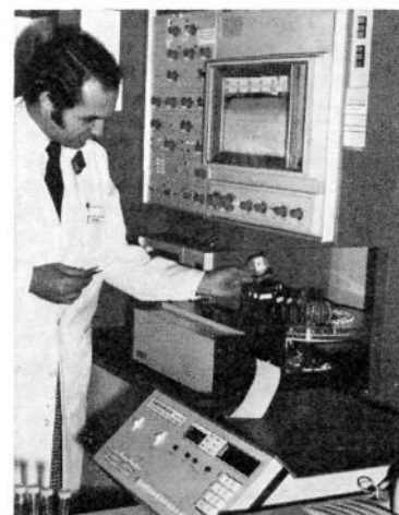
Dr. Farrell places a sample coil containing plasma from a newborn in an automated amino acid analyzer. Samples of 0.1 ml of blood or urine are processed automatically through ion exchange columns for measurement of all 21 common amino acids. Final results appear on printed tapes within 3 hours.
