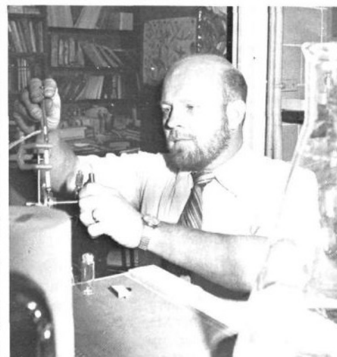
Using a high pressure liquid chromatograph, Dr. Jerina separates metabolites of polycyclic aromatic hydrocarbons in an attempt to identify those metabolites responsible for carcinogenic activity.
