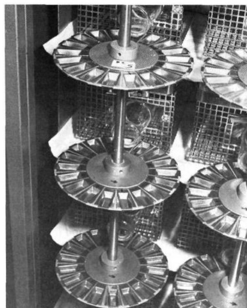
This Konig-Hofer feeding machine delivers test foods into animal cages at programmed intervals.
