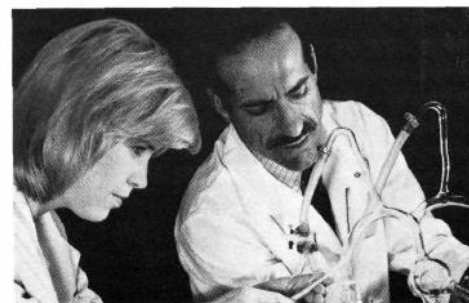
Testing for interactions of incompatible drugs, Clinical Center nurse Judith Lorette-Collins and BEIB engineer Dr. Robert Lutz infuse drug solutions through separate channels of a double-lumen catheter into a glass model of the human venous system (vena cava).
