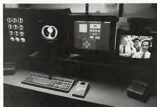
The Radiology Consultation WorkStation includes four monitors: two high-resolution black-and-white electronic view boxes (shown at left) for displaying radiographic images, a standard color computer display, and a high-resolution video monitor to show video signals from the collaborative site. A pan/tilt/zoom video camera, mounted atop the video monitor, sends images through the ATM network to other sites.
